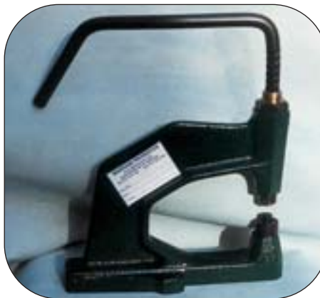
Manual lever press for eyelets, press studs etc.
