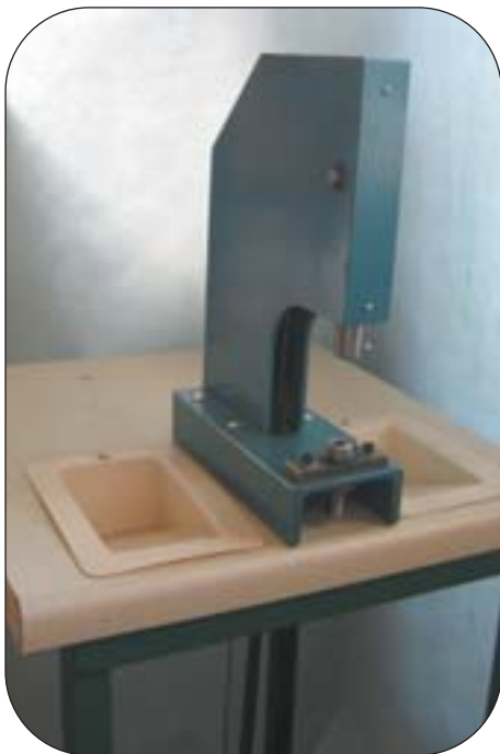
General purpose model with stand (many uses, foot operated) Different dies (tools) available.
