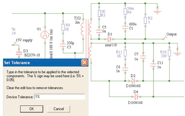
Monte Carlo analysis enables the engineer to simulate real life, where components operate within tolerance bandwidths. The percentage tolerance is entered and the circuit is simulated repeatedly with the component's operating tolerances automatically varied on each simulation run. The resultant compound waveforms enable the engineer to determine if the circuit still performs within design specifications when tolerances are varied.
