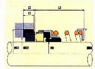
Basic rubber bellows style rotary available in a wide range of sizes to interchange with major brand seals & to suit DIN dimension pumps. Bellows assembly locates inside easily compressed parallel spring.
