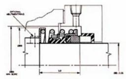
Generally marked 'CRANE' on rubber bellows. Bellows assembly locates inside robust parallel spring to give shorter working length but larger outside diameter.
