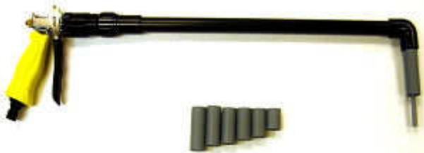
The total length of the filling pistol is 625 mm and it is supplied with a kit of eight spacer tubes so that the probe depth can be accurately set to suit the ranges of Alcad And Saft cells.
