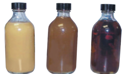
original emulsified oil after 1 month / 2 cartridge changes after 2 months / 4 cartridge changes
