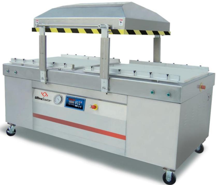
The Ultravac 1000's automatic lid swing function sets the pace for the packaging process maximising single operator productivity as they load product in one chamber while product is being sealed in the chamber at the opposite end. This Chamber Dimensions 45.2" x 43.1" (1148.1mm x 1094.7mm)
