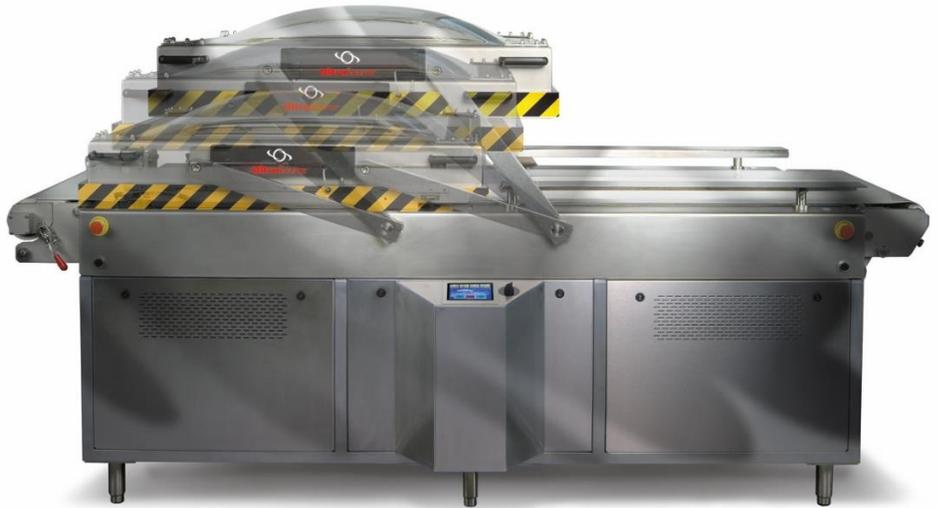
Designed to minimize floor space requirements, product is loaded onto one end of the seamless conveyor while the sealing chamber is in operation at the opposite end. The finished packaged product automatically moves from the sealing chamber to an off load conveyor or shrink tunnel while the loaded conveyor automatically moves into the sealing chamber and the process repeats.
