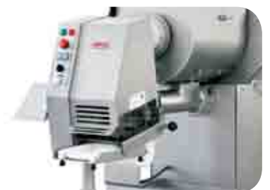
Pneumatic portioning device for minced meat on trays
