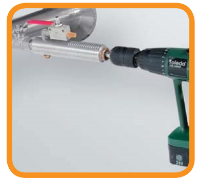
Drilling under pressure
