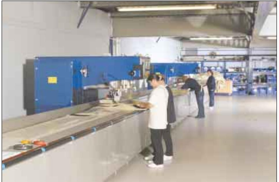
*Rubb's new 12 watt and 20 watt Fiab fabric welding machines insitu on the recently constructed mezzanine floor*
