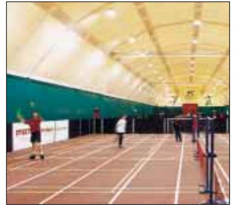
quickly erected by Rubb's site crews. The framework is then clad with an architectural membrane of PVC coated polyester. Ventilation can be provided along the entire length of the building. In addition Rubb can provide complete design integration with services, hard walls, side openings, netting and other systems.
