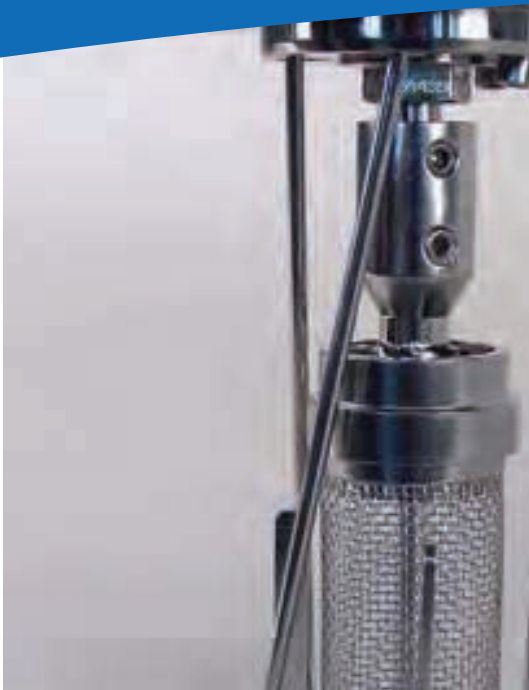
Spinning catalyst basket for 300ml / 350 bar reactor
