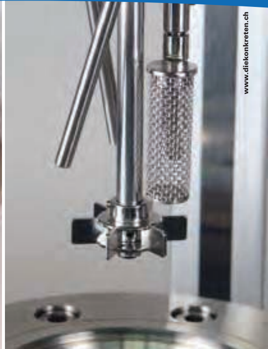
Fixed catalyst basket and turbine stirrer with gassing stirrer shaft for 1 liter / 60 bar reactor
