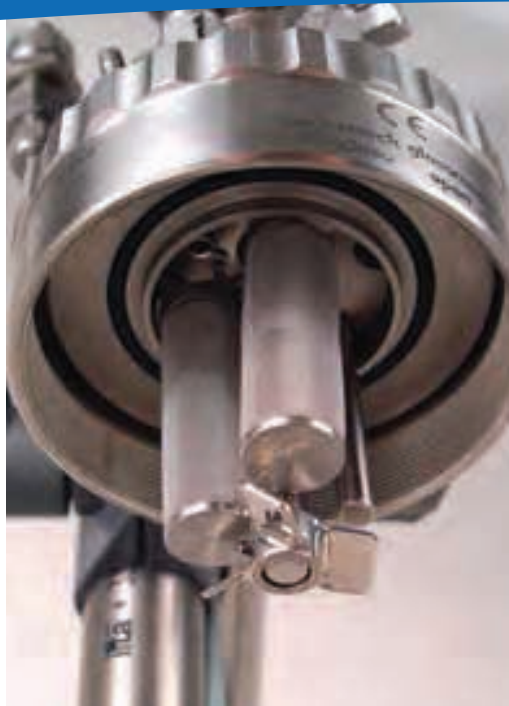
Double fixed catalyst basket with increased interaction surface for 200ml / 10 bar glass reactor
