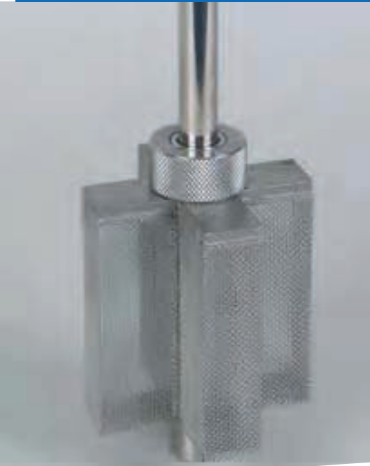
Spinning catalyst basket for 3 liters / 200 bar reactor
