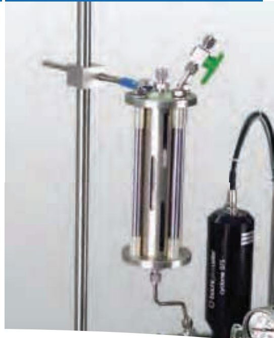
15 bar burette mounted on 3 liters pressure vessel
