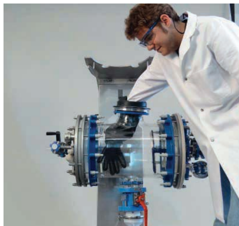
Removal of filter cake through containment system
