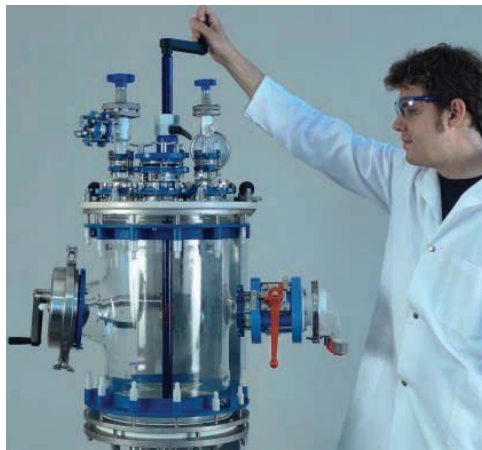
Height adjustable, glass lined stirrer
