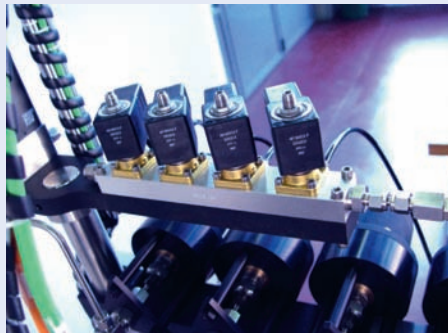
Manifold with control valves for massflow-controller
