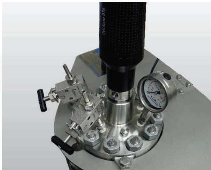
Reactor cover with numerous ports (probes, feed, etc.)
