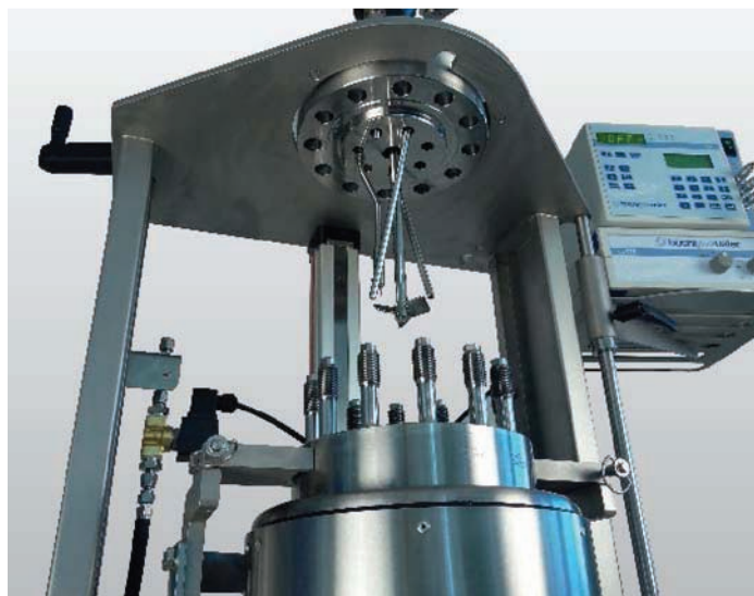
Reactor lift for easy cleaning and maintenance
