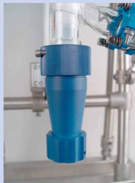
Flush-mount drain valve
