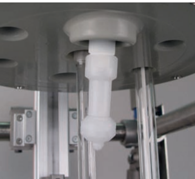
CIP spray head made of PTFE
