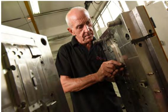
All our toolmaking is done by our inhouse toolroom. Due to the aggressive nature of magnetic material, good tool maintenance is key to the lifespan of the tool and quality of the components. Being able to offer this service in-house enhances the productivity of a magnet mould tool.
