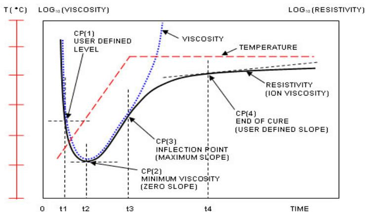
**Viscosity and resistivity in a curing material.**
