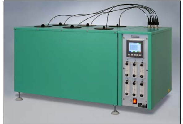
Cell Oven EB 19 , with 4 cells and individual temperature in each cell.
