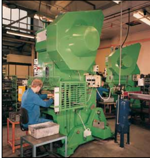
Open-fronted power press with light curtain
