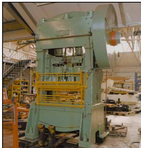
Typical interlocked guard
