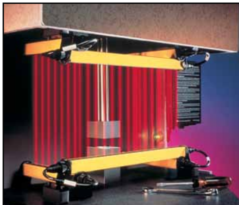
Minimum separation distance must be calculated to allow safe application of light curtain
