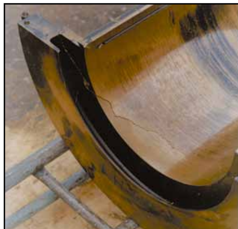
Severely cracked bearing
