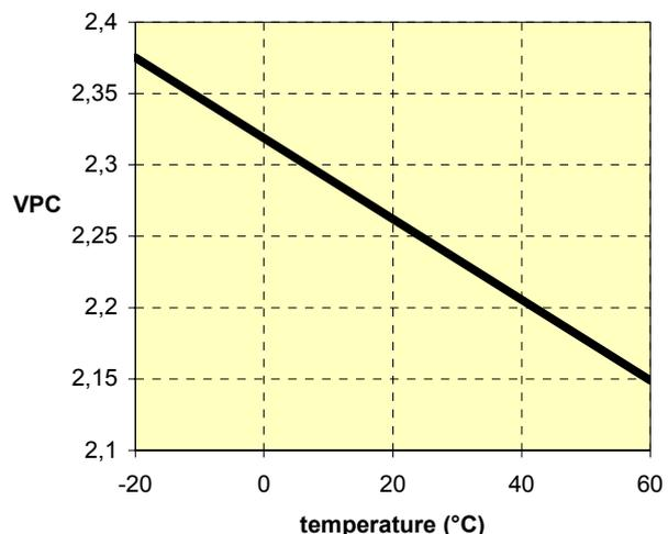
Fig. 5 Float Voltage vs. temperature
