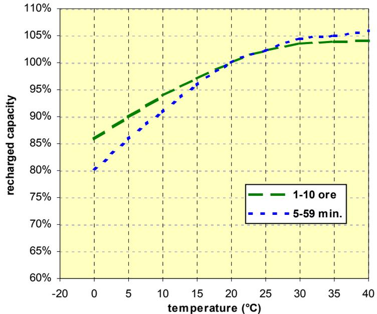
Fig. 4 Available capacity versus temperature
