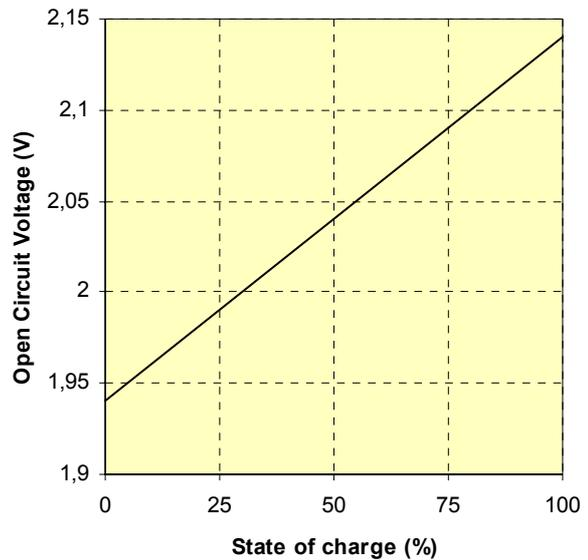
Fig. 3 Open circuit voltage in relation to the state of charge of the cell
