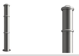
The GFC1500 Ornamental Mild Steel Bollard from AUTOPA is suitable for a wide range of locations and purposes. Constructed using mild steel, then galvanised to ensure its longevity. Cap and rings are welded onto the steel tube to complete the design.
