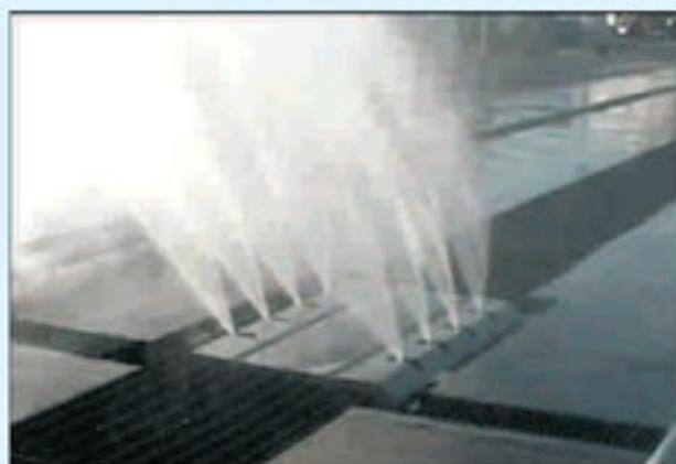
When washing smaller vehicles (e.g. passenger cars and vans), the pump of the outer sprays can be turned off due to the adequate coverage of the oscillating inner sprays.
