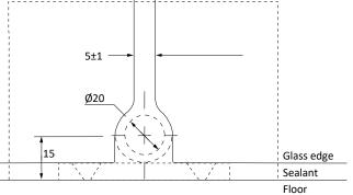
$Clamp \ \text{joining glass panels within glass flush with floor} \\$
