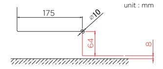
GCC would recommend the customer cuts 60mm depth (bottom gap 12mm) to allow for most floor condition.
