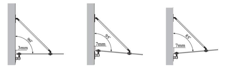
The slope of the Glass Canopy can be adjusted +/- 5° by revolving the connecting rod.
