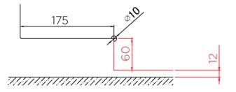
There are two different glass cut outs for the HGT-100, resulting in different bottom clearances.
