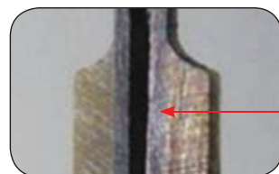
The needle and hub are permanently fused, greatly increasing the strength.
