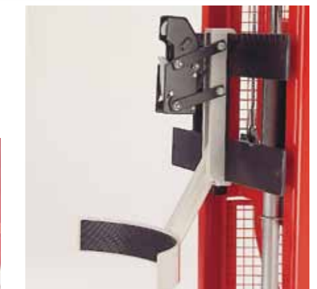
Drum Claw Max load: 250 kg. For transporting of 210 litre tight head drums at low level only Ref: MSU 5 15
