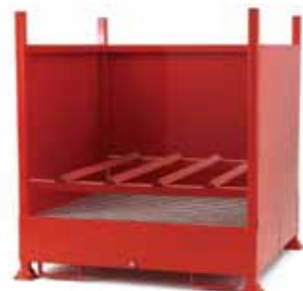
DS406 Drum sump with back and 2 sides for 2 horizontal drums - 470 ltr capacity sump. Stackable 3 high o/a L x W x H: 1440 x 1440 x 1500mm
