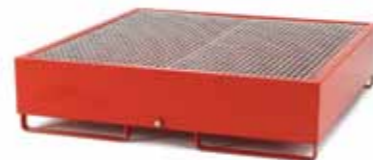
DS402 Drum sump for 4 vertical drums - capacity 470 ltrs removable galvanised steel support grid o/a L x W x H: 1365 x 1365 x 345mm
