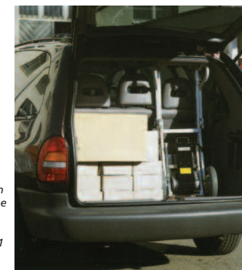
Compact: With its handles that can be pushed into the frame and the thus comparatively small size of the CargoMaster C141 Vario, it finds room in even small vehicles.
