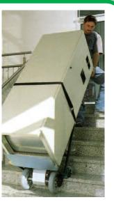
The CargoMaster A 310 has been specifically designed for the transport of heavy loads such as heating boilers, stoves, heaters or parts of machinery. Thanks to its powerful 24 volt electric drive, it masters up to 310kg effortlessly. The fortified frame of the A 310 as well as its toe plate, adjustable in height, make allowances for the extreme demands on the machine.
