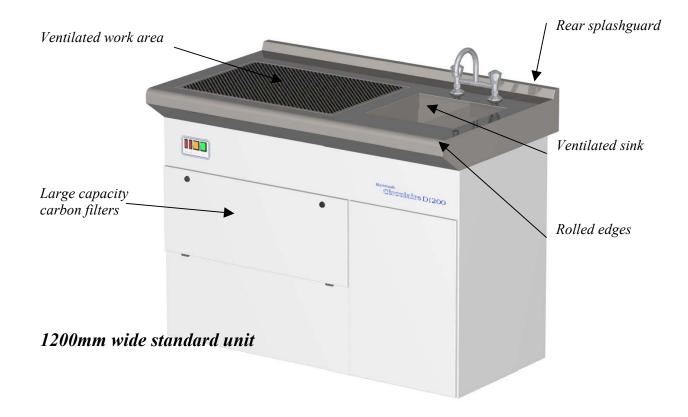
Units are constructed for maximum reliability and strength. All worksurfaces are manufactured from 316-grade stainless steel whilst the lower section is manufactured from zintec powder coated steel to prevent corrosion (If preferred, lower section can also be manufactured from stainless steel).
