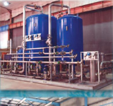
Demineralisers use both cation and anion resin to remove dissolved solids in the water. The cation resin must be regenerated using acid and the anion resin using caustic or brine
