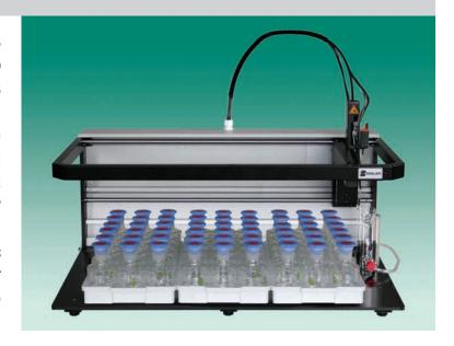
For the BOD application the SP50 Robotic Analyzer accommodates 54 bottles, divided over 3 separate racks of 18 bottles each. The SP50 offers a complete "walk-away" automated BOD concept, including automatic addition of dilution water to the BOD bottles, automatic addition nitrification inhibitor (ATU) and automatic seeding. Furthermore the SP50 analyzer can also be equipped with a second oxygen probe for increased sample throughput by analyzing two samples simultaneously.
