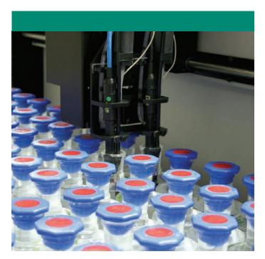
Besides the automation of BOD, a variety of other applications can be automated on the SP50 Robotic Analyzer such as pH, EC, Turbidity, Color, ISE, alkalinity and others.
