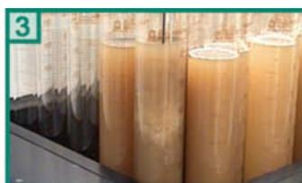
**3** Automatic addition of dilution water to volume and stirring of the sample
