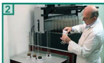
**2** Place the sample into the cylinder and add 50 ml of Sodiumpyrophosphate
