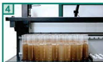
**4** Settling time, normally between 4 and 8 hours for 2 µm particles
