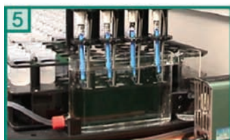
5 Between each operation the SP1000 rinses the probe
