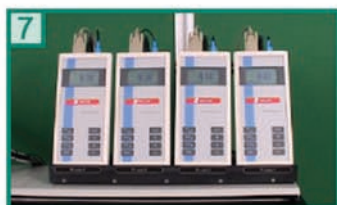
7 After stirring the pH value of each sample is measured
