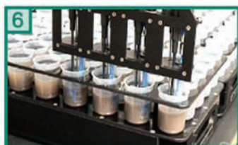
6 After a pre-defined settling period the samples are again stirred
