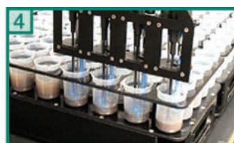
4 The SP1000 adds extraction solution and stirs all the samples in sets of four
