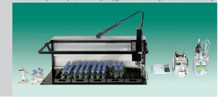
Accurately controlling the quality of drinking water has become increasingly important. The condition of the source water from which it is drawn and the treatment it receives varies greatly from one location to another. The Skalar SP1000 Robotic Analyzer was designed specifically for monitoring this process.
