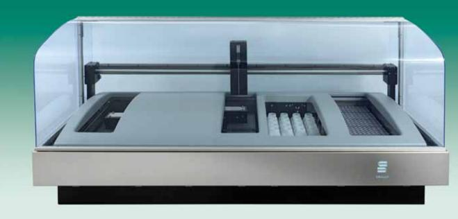
The BluVision<sup>™</sup> analyzer is designed to perform colorimetric analysis for the environmental field, with optimal ratios of sample and reagent volumes to achieve lower detection limits with high accuracy. By increasing the path length of the disposable cuvettes, the system offers much lower detection limits and a broader linear range than any other current discrete analyzer.
