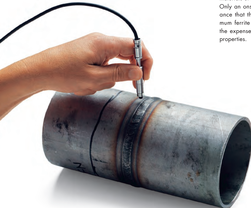
Measurement of the ferrite content of a weld seam
