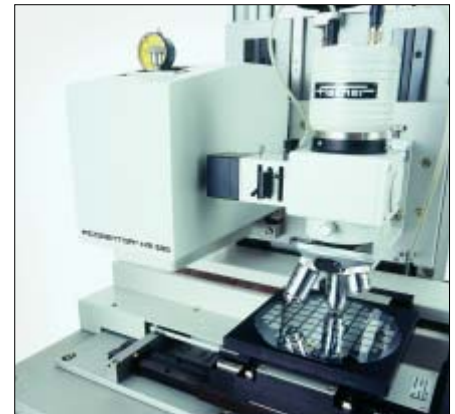
Coated wafer as the specimen under the video microscope for the accurate determination of the measurement position(s).
