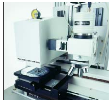
To make measurements, the measuring stage travels automatically under the measuring head such that the hardness indentations occur exactly at the selected measurement positions.
