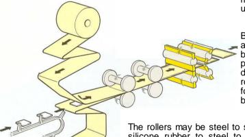
Both webs pass over separate tension arms, which operate the respective reel brakes. The product is fed at the correct pitch between the two webs, which are drawn from the reels by two sets of rollers in tandem. Each set consists of four rollers; one upper and one lower at both edges of the web.
