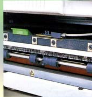
Type 80 Statstrip used to reduce static build up on paper processing.
