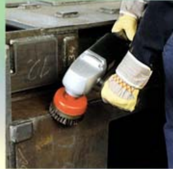
A cup brush and angle grinder at work.
