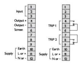
As with single width units, the 'screen' terminal is not necessarily connected to earth but does provide a convenient earth bonding point.
