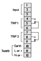
From the above, it may be seen that a single trip has double pole relay contacts wired out while a double trip has single pole contacts per trip.
