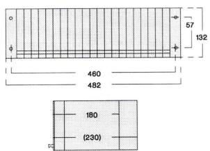
Racks should not be mounted closer together than 485mm horizontally or 135mm vertically. They would normally be mounted further apart than this for ease of wiring. At least 180mm must be left at the front of the rack to allow for module withdrawal.
