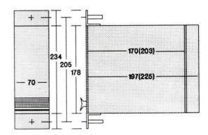
A 65mm wide by 190mm high aperture must be cut in the front panel with 6mm fixing holes above and below. The brackets and front panel are wider than the aperture to obscure any cut edges.
