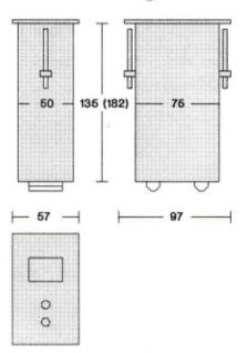
The second option is very similar to the above but is designed for panel mounting. This has a 57mm X 97mm front panel and the leaf type terminal blocks are mounted at the rear of the unit. These blocks will also accept cables up to 2.5mm².
