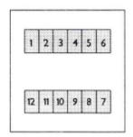
When viewed from the rear, the terminals are numbered clockwise from the top left rather than anti-clockwise from the top right.
