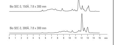
Separation of E. coli lysate on 150Å and 300Å Agilent Bio SEC-3 HPLC columns. The smaller pore size 150Å column provides better resolution of smaller proteins.
