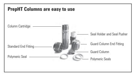
PrepHT cartridge columns have a unique design that makes them easy to install and seal finger-tight up to 5000 psi. The cartridge design allows for an integral guard column to be used, which prolongs the life of the purification column. This cartridge configuration is economical to use since the column cartridge and/or the guard cartridges are replaced independently. The end fittings are used many times.
