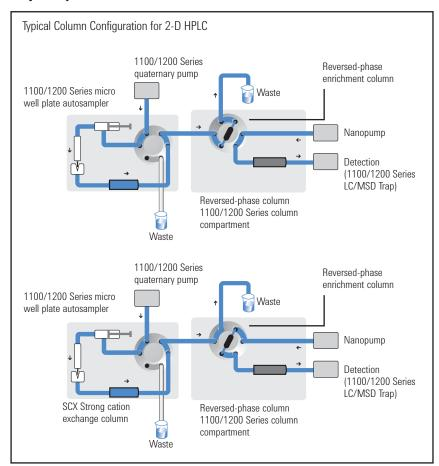
Flow path of the Agilent 1100 Series Nanoflow Proteomics Solution system.
