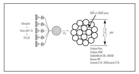
Figure 1. Formation of ZORBAX porous silica particles
