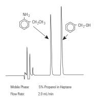
Figure 3. Chromatographic improvement using highly purified ZORBAX Rx-SIL
