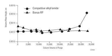
Triple endcapping of Bonus-RP enhances stability at pH 7. Each 10,000 column volume is equivalent to approximately one working month.
