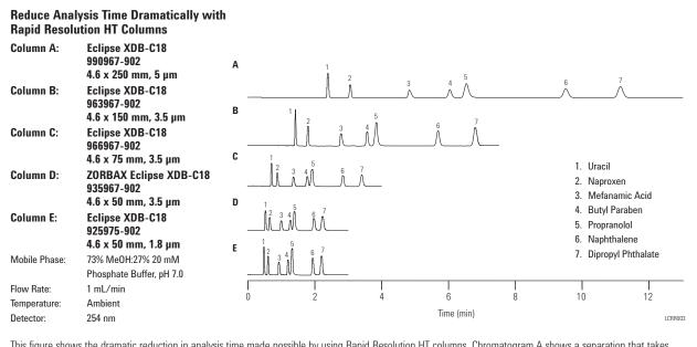
This figure shows the dramatic reduction in analysis time made possible by using Rapid Resolution HT columns. Chromatogram A shows a separation that takes 11.5 minutes on a 25 cm, 5 µm column. Rapid Resolution (3.5 µm) columns, shown in chromatogram B and C, reduce analysis time substantially, but with a slight compromise in resolution. The Rapid Resolution HT column reduces analysis time to 2.2 minutes, an 80% reduction, while still maintaining baseline resolution.
