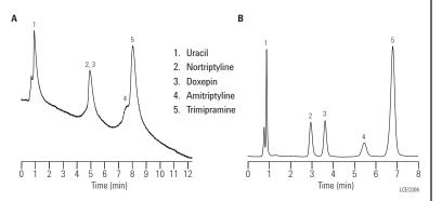
Double endcapping, dense bonding and the durable Rx-Sil particles (sol-type) combine to provide long lifetime at pH 7 when compared to single endcapped sil-gel columns used here. The conditions used for this test — high temperature (60°C) and high salt concentration (250 mM), accelerate the dissolution of silica, causing premature failure of the sil-gel type column.
