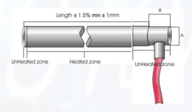
TYP 9 nipple Choice of sheath material: stainless steel 0,02-0,06mm
