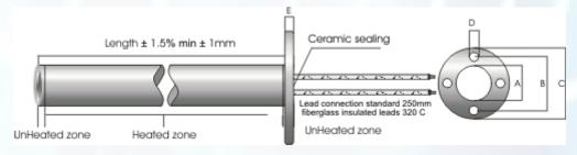
TYP 8 cilinder Choice of sheath material: stainless steel 0,02-0,06mm
