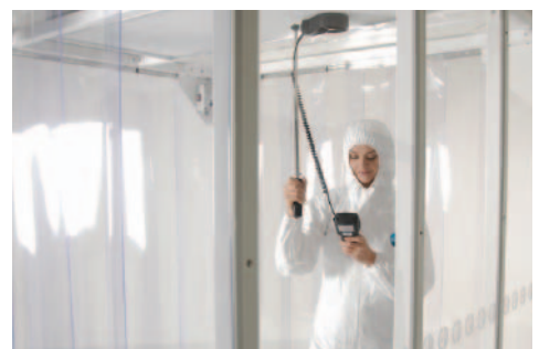
Above: Air velocity measured using rotating vane anemometer.
