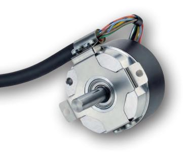
The AD34 is the most compact absolute encoder in class. It is available with a resolution up to 17 Bit Singleturn. The mechanical design consists of two ball bearings and a flexible torque support. The AD34 complements the ACURO-DRIVE series and is appropriate for use within BLDC servo motors with small frame sizes. The AD34 is available with a notched shaft, which saves installation time.
