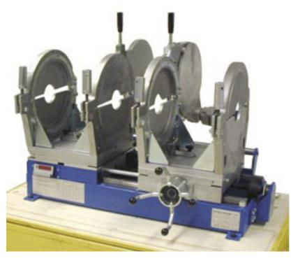
For fusion jointing PP, PE and PVDF pipes and fittings for accurate single or series prefabrication of fitting (segment bends d 90 - 315 mm)
