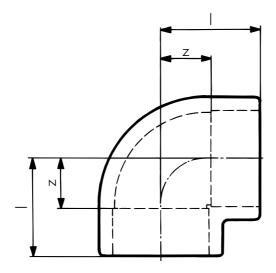
Fitting with outer joint end
