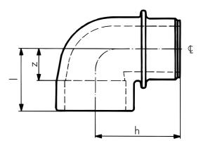
Inner joint ends are referred to as **sockets** and outer joint ends as **spigots**.
