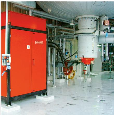
To maintain the agitator shaft sealings the lightweight compact hydraulic motor is removed with hoses still in place making the procedure simple and much quicker than normal. Full variable speed adds flexibility to the process.
