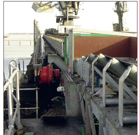
This Amco Birtley belt conveyor is 200m long with speed range up to 2.5m/sec and capacity of 3000 tonne/hr of coal from the ship unloaders. Smooth dynamic acceleration and braking is available with loaded conveyor to stop quickly to prevent flooding the downstream conveyors.
