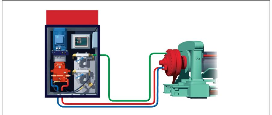
A typical Hägglunds Drive consists of a drive motor selected from the wide range available to give the torque required. A power unit with a variable displacement pump/motor set and necessary tank, filters and instrumentation. A control and monitoring unit and the inter piping. The arrangement is versatile and flexible which enables customisation to suit the exact requirements of the application and environment.
