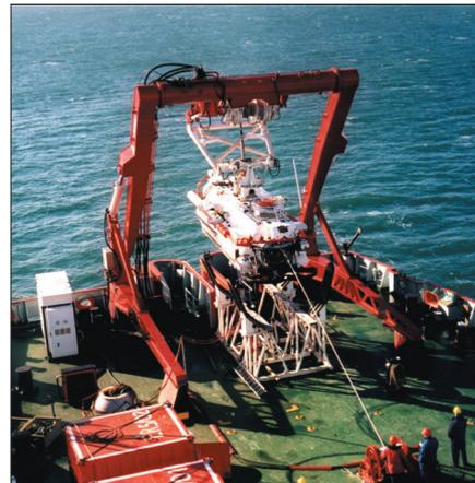
This SMD submarine rescue vehicle launch system uses Hagglunds Viking motor and brake at the winch for superb tension control and the Hagglunds power unit stands close by.
